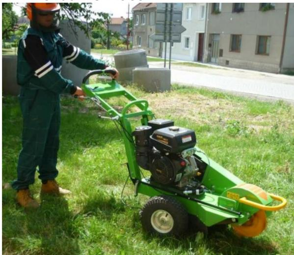
While working, the attendant should stand behind the grip (see fig.), holding it with both hands and with both feet standing on a flat and firm base. All working motions should be continuous and uniform.
