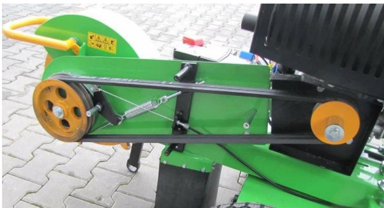
**!** For proper belt tension check up also alignment of pulleys (their faces) starting as from the belt pulley put on the shaft together with the cutting head. This shaft is bedded in two fixed bearing housings. Before adjustment, check up also proper bedding of pulleys on the shaft (tongue and groove). Each pulley must bear on the shaft shoulder and be fixed by its central fixing bolt (torque 80 Nm).
