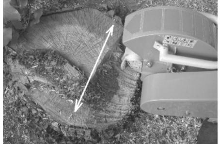
Stump cutting in layers at swinging motion
